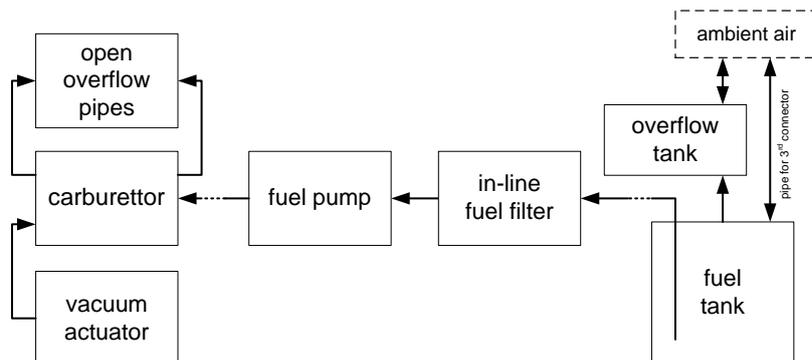
↳ *Since the beginning of 2010 we have started using a new rectangular fuel pump instead of the round Mikuni fuel pump. The advantage of this pump is that it has an internal pressure limiter. Therefore it is no longer necessary to install a return to the fuel tank, and the needle valve of the carburettor has better performance.*
